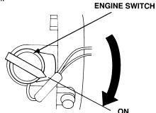
Figure 10. Engine ON/OFF Switch (ON Position)
